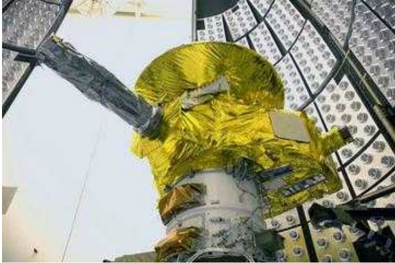
Figure 2. The 1060-pound New Horizons Spacecraft in the Payload Hazardous Servicing Facility at the Kennedy Space Center, Florida, was launched on 19 January 2006 and is due to approach Pluto on 14 July 2015. It carries seven scientific instruments including the powerful Long Range Reconnaissance Imager (LORRI) camera.
